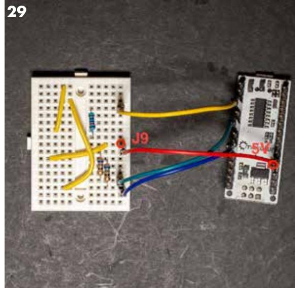
Use a fourth jumper wire to connect the 5v power from the nano to the LED. This will go from the 5V pin, fourth up from the acrylic on the right of the nano, to the J9 hole on the breadboard.
