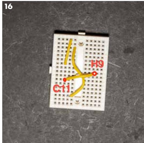
Cut another 1 1/4" section of the wire and strip its ends. Push this one into H9 and C11.
