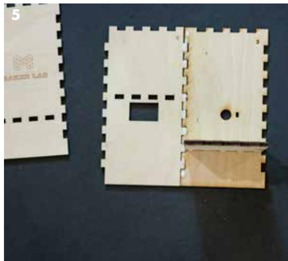
Also glue in the rectangular piece with a small notch cut out of one side - notch to the right.
