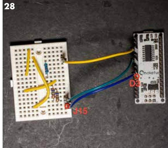
Use another jumper wire to connect D3 (3 pins down from D6) on the nano to J15 on the breadboard. This is the blue LED pin.
