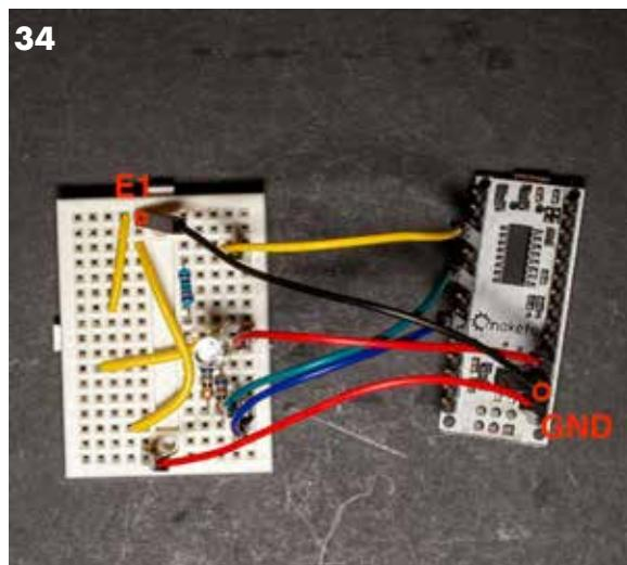
Connect the ground GND on the nano to E1 on the breadboard and A0 on the nano to C9 on the breadboard.
