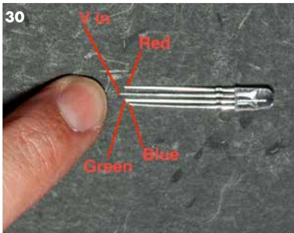
The long pin on the LED is the power (V) the one above it is red the two below are green and blue. Bend the long pin so that it matches the length of the others. All four pins go into the breadboard at once.
