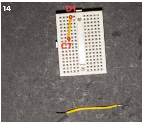
or wire strippers to remove the sheath from 3/16" of the wire. Push one bare end of the wire into D1 on the breadboard and the other end into C7.
