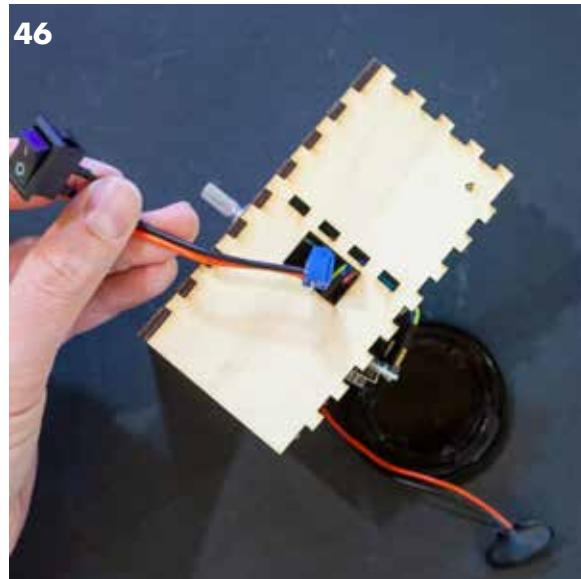
Slide the switch terminal block through the large rectangular hole.
