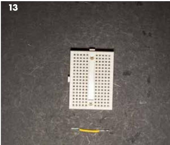
Lay the box aside to dry and get out the electronics. Cut a roughly 1 1/4" piece of the solid core wire. (There is only one in the kit color does not matter.) Use a pair of scissors
