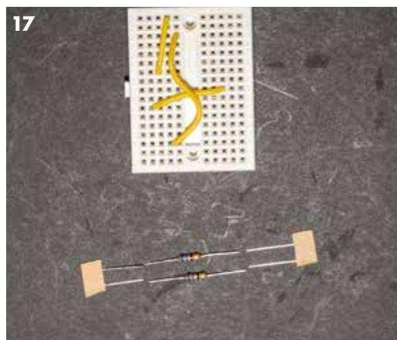
Take the two resistors that are connected and cut them down to about a 1/4" from each side of the resistor. Bend the ends at a 90 degree angle.
