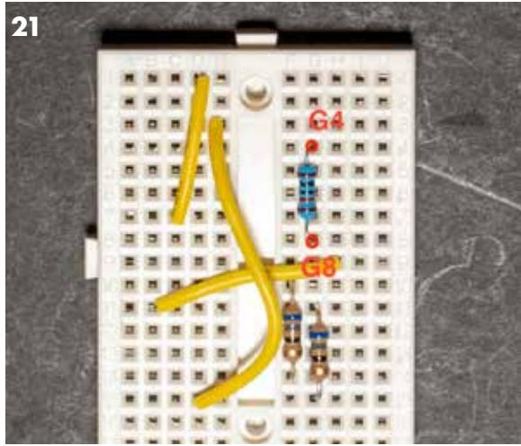
Push the last resistor into G4 and G8 on the breadboard.
