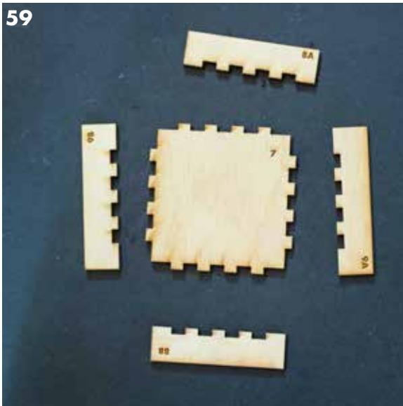
To make the end cap arrange pieces 8A and 8B above and below pieces 7 with 9A and 9B
