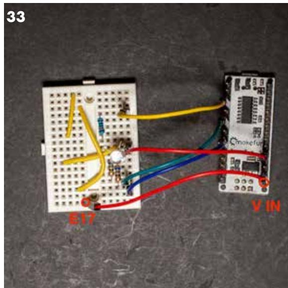
Use a jumper wire to connect the power in V IN on the nano to E17 on the breadboard.
