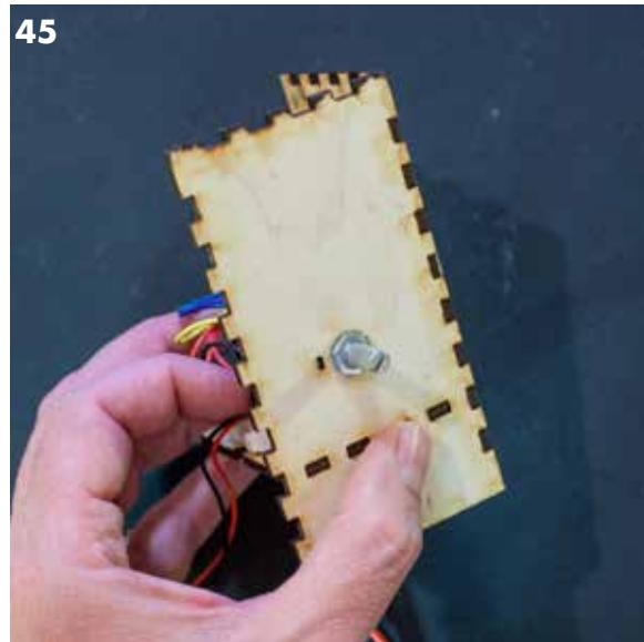
Place the washer on the post from the outside then tighten the nut onto the post also.
