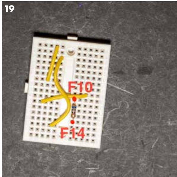
Push one end of one resistor into F10 on the breadboard and the other end into F14.
