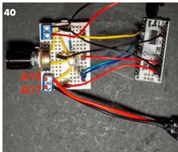
Plug the Switch terminal block into holes A15 and A17. Connect a 9v battery and test before continuing to put the electronics in the box.
