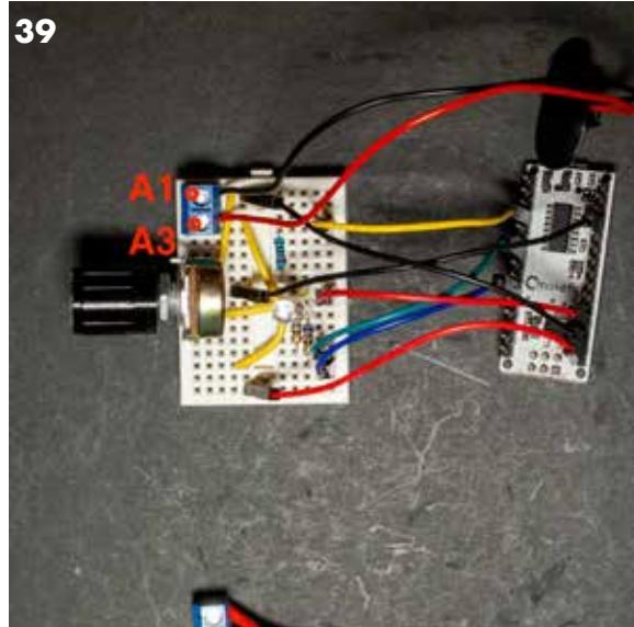
Plug the 9v battery adapter terminal block into holes A1 and A3 on the breadboard.
