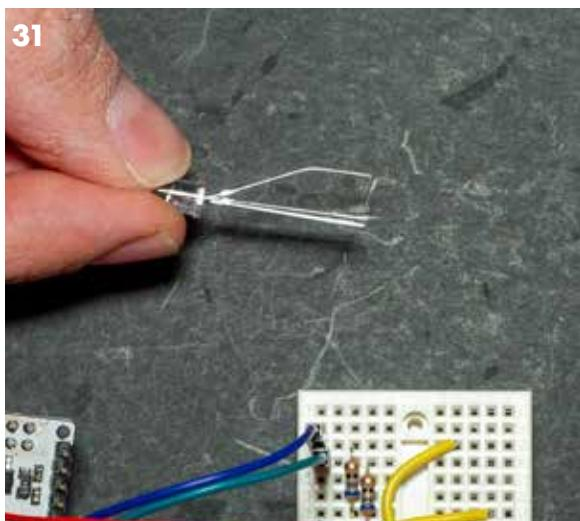
Red goes into I8. The long power pin goes into F9. Green goes into I10 and blue goes into hole I11.
