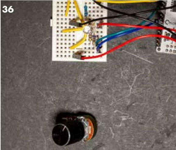
Take the potentiometer and remove the knob. It pulls off with effort. Then unscrew the nut and remove the washer.
