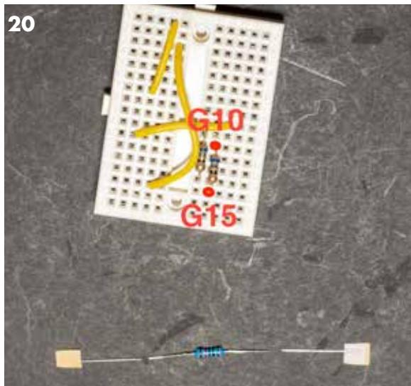
Put the other resistor into G10 and G15 on the Breadboard and cut the single resistor like the other two.
