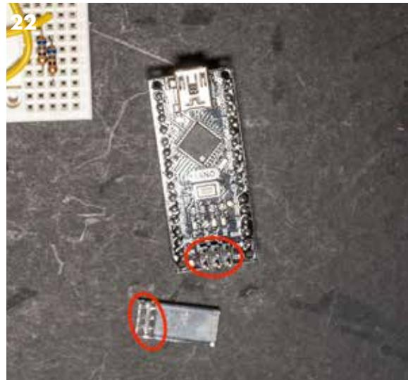
Take out the Arduino Nano and the small piece of acrylic. Press the 6 pins on the back of the nano into the 6 holes in the acrylic.
