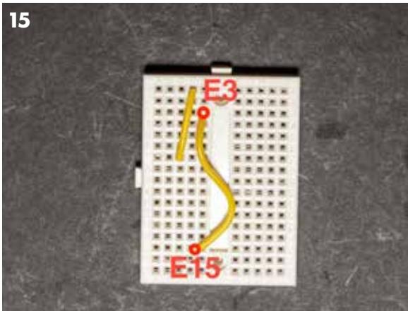
Cut a 1 3/4" section from the same wire and strip its ends. Push those ends into E3 and E15 on the breadboard.
