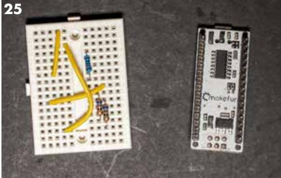
Flip over the nano so the majority of its pins stick up. Use the female end of a jumper wire to connect pin D9 on the nano, the fourth down on from the USB port on the left. Connect the male end of the same wire to J4 on the breadboard. This will be the red RGB LED connection but colors don't matter.
