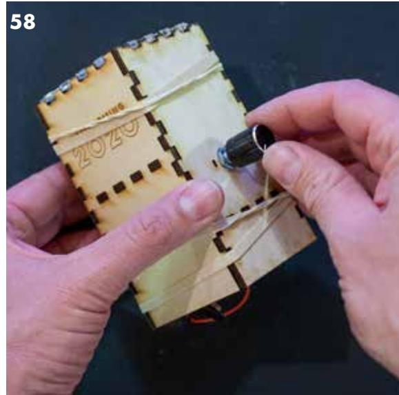
Push the knob back onto the potentiometer post.
