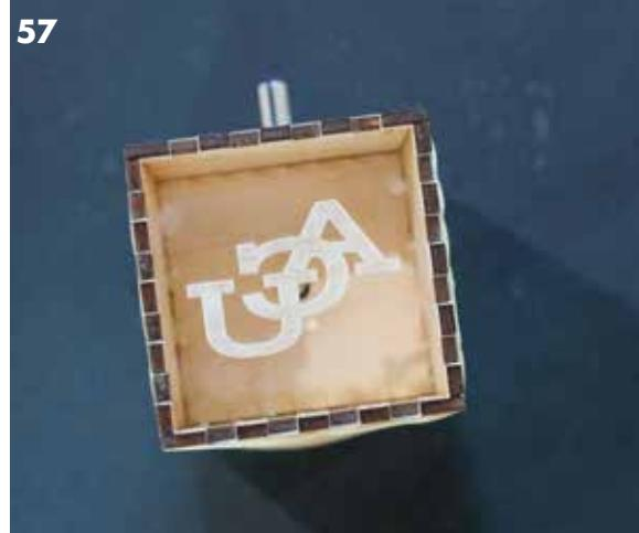
The ACU logo acrylic should be put on backwards so that it casts a shadow the correct direction. This can be glued between the finger joints.
